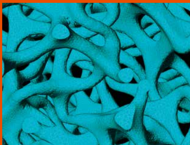
Attention to detail: A finite element mesh of an open-cell foam.
