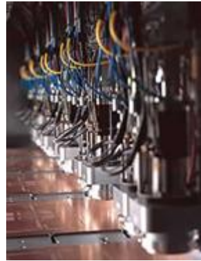
Air Bearing Spindles being used to Manufacture Printed Circuit Boards
